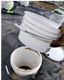
2. Collar is made by cutting bottom half of 5 gallon bucket and placed inside lower bucket.
