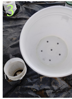
3. Upper bucket has drainage holes with 250µm nylon mesh glued over them to prevent escape.
